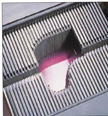
Figure 1. Multileaf collimators. Each of the 5 mm “leaves” has its own small motor and they continually move to create the dose distribution.
