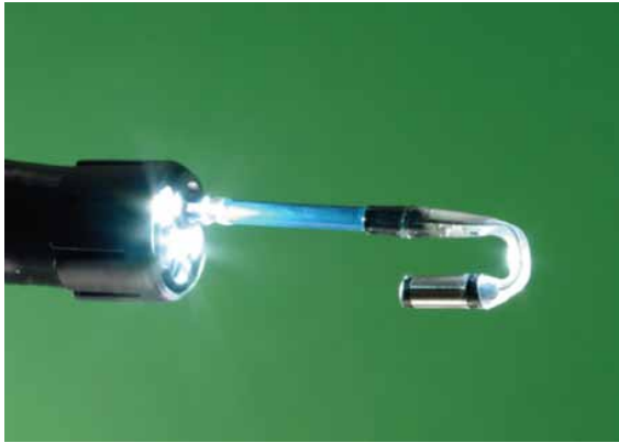
Figure 1. The Third Eye Retroscope automatically turns 180 degrees when extended from the instrument channel of the standard colonoscope. A miniature video camera is housed in its tip and provides a continuous retrograde image during withdrawal through the colon. The light-emitting diode in the bent portion of the instrument provides illumination for the camera. A polarized hood on the tip of the colonoscope prevents the bright light emitted by the retroscope from interfering with the automatic iris of the colonoscope.
